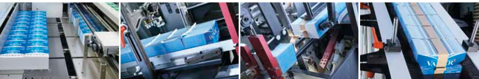
Strip feeding, stack separation, banding, output: the new machine concept allows complete processing, from strip stacks to label bundles.
